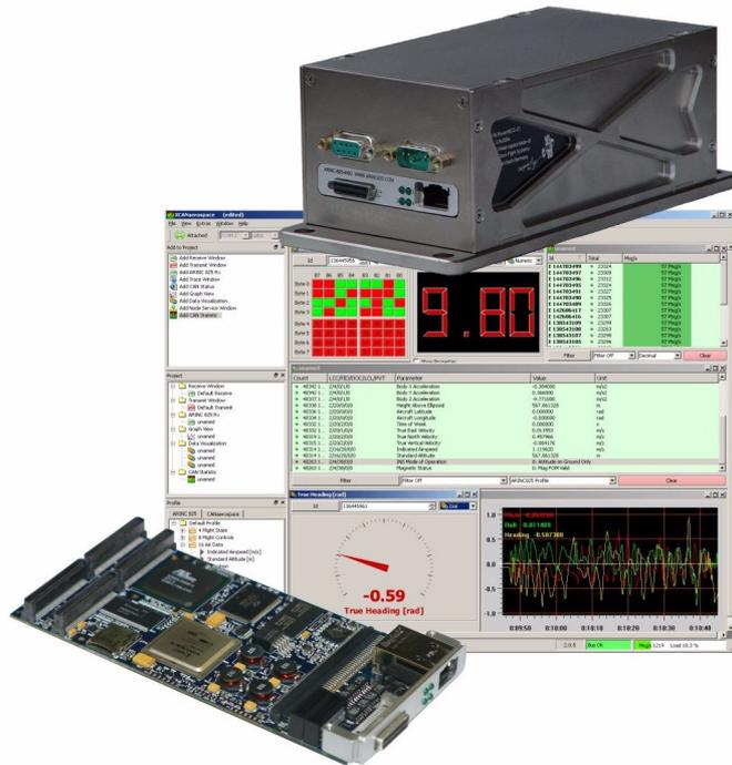
The PMC825 system includes a PMC format module supporting 4 fully independent, optically-isolated ARINC 825 channels or 8 fully independent non-isolated ARINC 825 channels. Each module also contains a 10/100/1000 BaseT Ethernet interface and a Bus Mastering PCI interface operating at up to 64 bits and 66 MHz for data exchange to the host platform.
